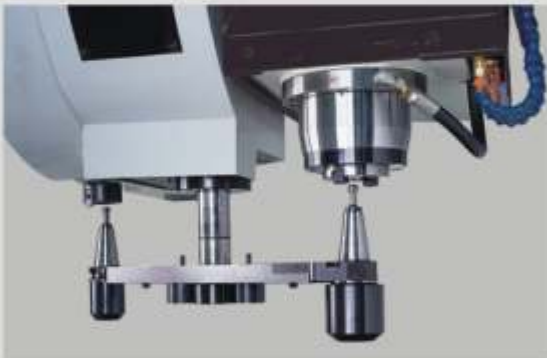
➤ ARM TYPE QUICK TOOL CHANGER (OPTIONAL) Tool to tool 2.5 secs
