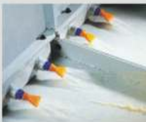
➤ High pressure water jet for chip removal
