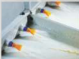
➤ High pressure water jet for chip removal
