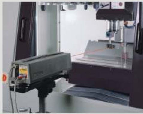
↘ LASER INSPECTION SYSTEM All 3 axes are checked by Laser test to ensure positioning and repeating accuracy.
