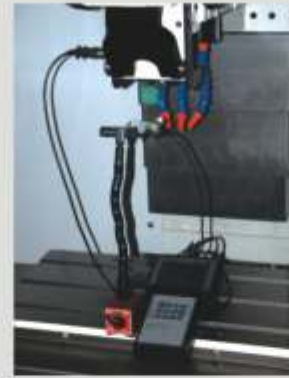
↘ SPINDLE NOISE&VIBRATION CHECK
