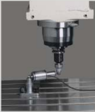
↘ BALLBAR TEST Every machine is inspected by Ballbar test to ensure machining accuracy.
